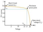
When the load is short circuited, maximum current flows and is called Isc, short circuit current. When the load is open circuited we get the point on the x-axis of maximum voltage Voc, open circuit voltage. In both the above cases power
