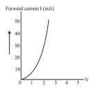
The I-V characteristics is very similar to a forward biased p-n junction diode.
