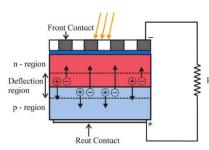
positive side (n-side) and holes to the negative side (p side). These carriers generate voltage and hence power the external load.
