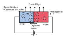
The diode being forward biased, the electrons in the conduction band recombine with the hole in the valance band and the energy released in the form of light. It is made in
